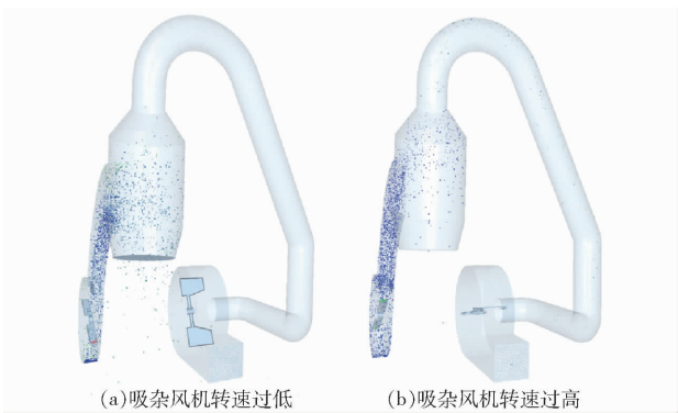
图 8 吸杂风机转速过低、过高时清选系统内胡麻脱粒物料的运动情况 Fig. 8 Separation and cleaning state of two kinds of impurity suction fans with improper speed
