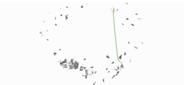
图 16 A* 算法在规划图层路径规划 Fig. 16 A* algorithm in planning layer path planning
