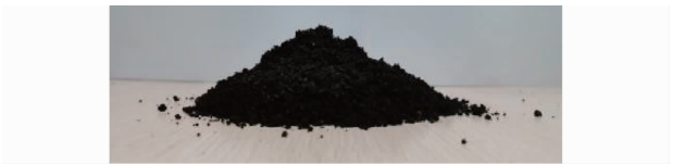
图 1 自然休止角测定 Fig.1 Determination of natural angle of repose
