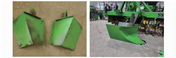
(a) 板式起垄装置 (b) 犁铧式开沟起垄装置 图 15 板式和犁铧式开沟起垄装置 Fig. 15 Ridging shaping device of plate type and ploughshare ridging shaping
