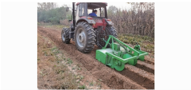
图 14 甘薯起垄整形机田间试验 Fig. 14 Field experiment of sweet potato ridging shaping machine
