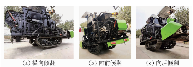
图 12 整机静态倾翻试验 Fig. 12 Static tipping tests of whole machine
