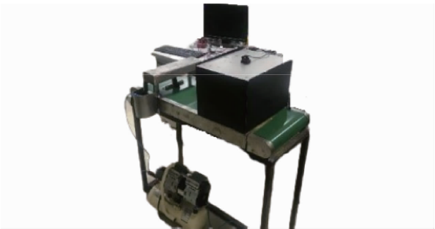
图 12 霉变玉米种子实时检测分选样机 Fig. 12 Detection and sorting device for mildew corn seeds
