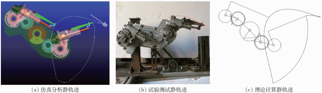
图 11 移栽机构静轨迹对比 Fig. 11 Comparison of relative movement trajectories of transplanting mechanism
