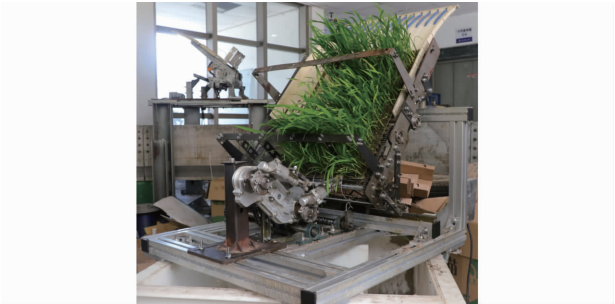
图 12 夹钵式水稻钵苗移栽试验台 Fig. 12 Rice bowl seedling transplanting test stand with bowl type
