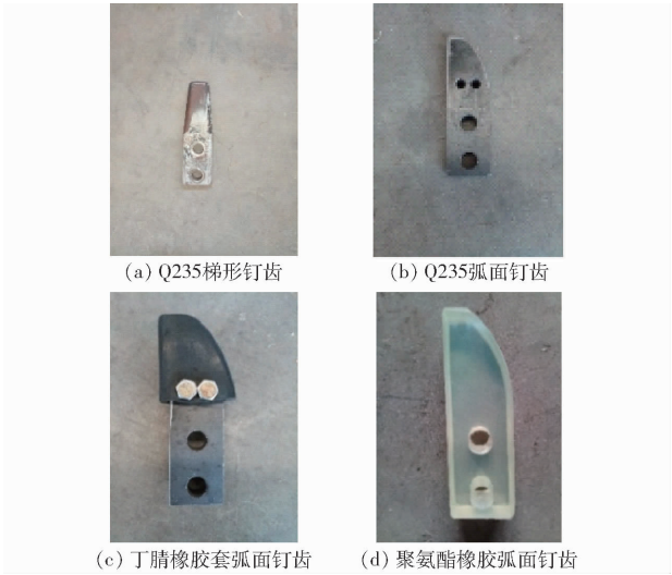
图 8 脱粒钉齿 Fig. 8 Types of spike-tooth
