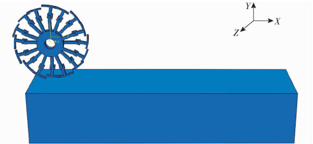
图 7 仿生步行轮/土壤相互作用模型 Fig. 7 Interaction model between bionic walking wheel and soil
