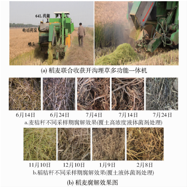
图 7 稻麦联合收获开沟埋草多功能一体机及作业效果 Fig. 7 Harvest ditch and stalk-disposing machine and its operation effect
