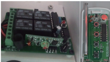
图 8 卷帘电路控制板和无线按键控制器 Fig.8 Diagram of circuit control board and wireless key controller
