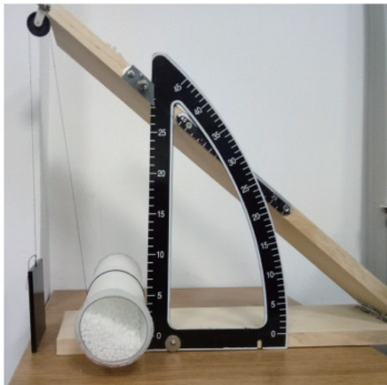
图 9 倾斜法休止角测定试验 Fig. 9 Test of measuring angle of repose by tilt method
