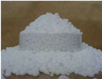
图 11 分体圆筒法休止角测定试验 Fig. 11 Test of measuring angle of repose by split cylinder method
