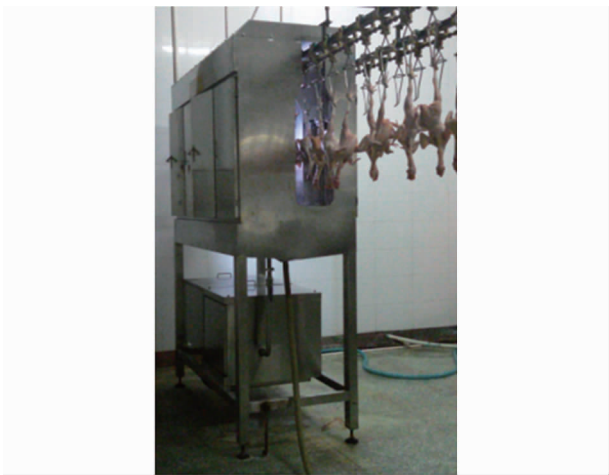
图8 鸡胴体表面污染物在线检测及处理系统实物图 Fig.8 Photo of online detection and processing system for contaminants on chicken carcass
