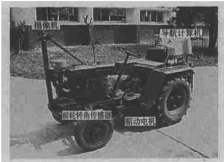
图 2 机器视觉导航农用轮式移动机器人原型 Fig. 2 Prototype of agricultural wheeled mobile robot navigated based on machine vision
