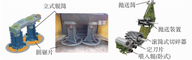
图 16 自走式灌木平茬收割机割台及切碎装置示意图 Fig. 16 Schematic of cutting head and chopping device of self-propelled shrub harvester
