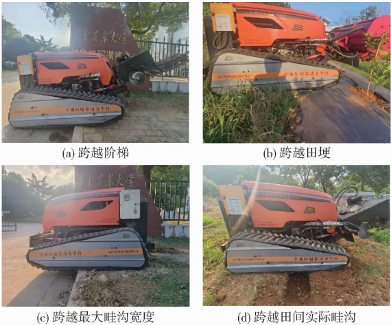
图10 越障试验 Fig.10 Obstacle tests
