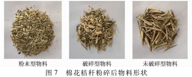
Fig.7 Material shape after crushing of cotton straw
