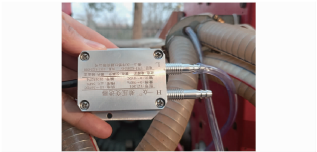
图5 差压变送器及负压输送头连接方式示意图 Fig.5 Diagram of differential pressure transmitter and negative pressure delivery head connection method
