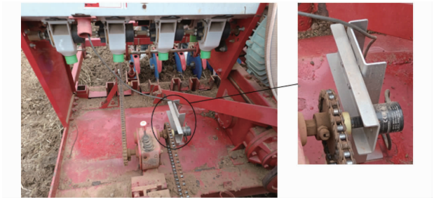
图6 地轮编码器装配图 Fig.6 Diagram of ground wheel encoder assembly
