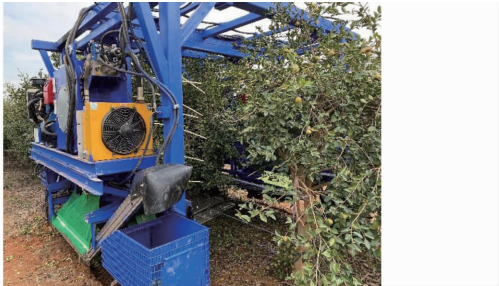
图 15 履带式高地隙油茶果振动采收机作业试验 Fig. 15 Orchard test of crawler-type high clearance Camellia oleifera fruit vibratory harvester
