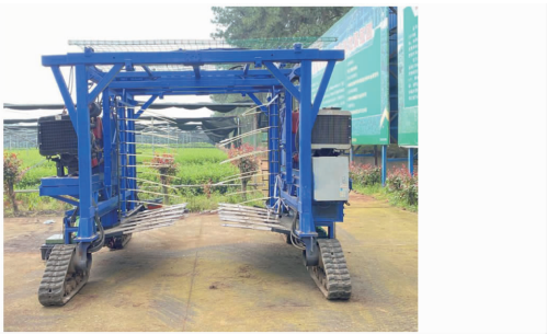
图 13 履带式高地隙油茶果振动采收机实物图 Fig. 13 Photo of crawler-type high clearance Camellia oleifera fruit vibratory harvester
