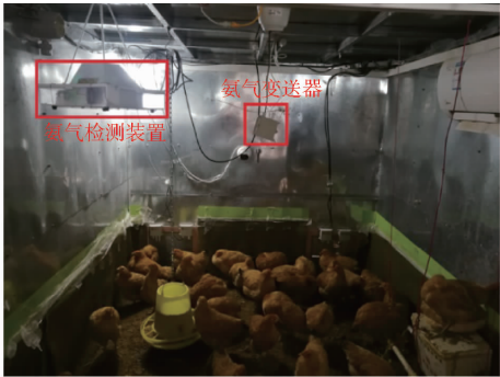
图 11 现场试验 Fig. 11 Ammonia detecting test in broiler chamber
