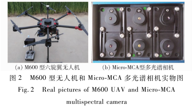
图 2 M600 型无人机和 Micro-MCA 多光谱相机实物图 Fig. 2 Real pictures of M600 UAV and Micro-MCA multispectral camera
