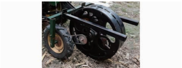
图 11 滚筒式免耕播种机构样机功能试验 Fig. 11 Function test of drum-type no-till planter mechanism
