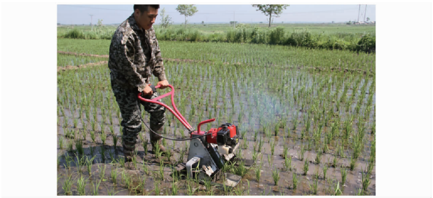
图 6 双行水田除草机田间作业性能检测 Fig. 6 Performance test of double row paddy field weeding machine in field
