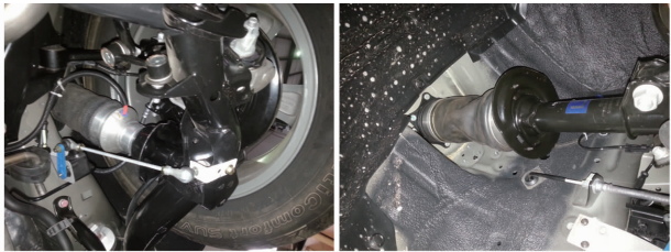
图 1 改装后试验车辆的前悬架、后悬架 Fig. 1 Modified front and rear suspensions of experimental SUV
