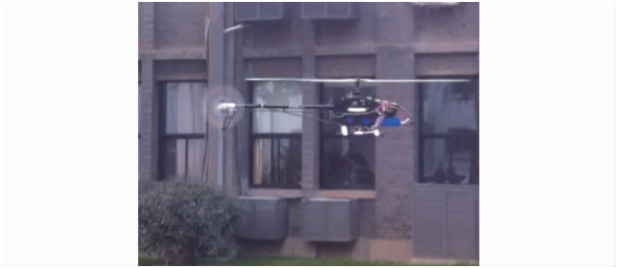
图 7 Trex-600 型无人直升机航向轨迹跟踪实验 Fig. 7 Yaw angle trajectory tracking test of Trex-600 unmanned helicopter
