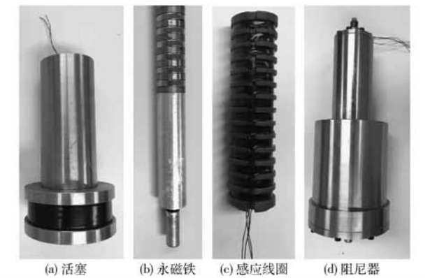
图 8 功能集成型磁流变阻尼器关键元器件与样机 Fig.8 Key parts and prototype of multi-functional MR damper
