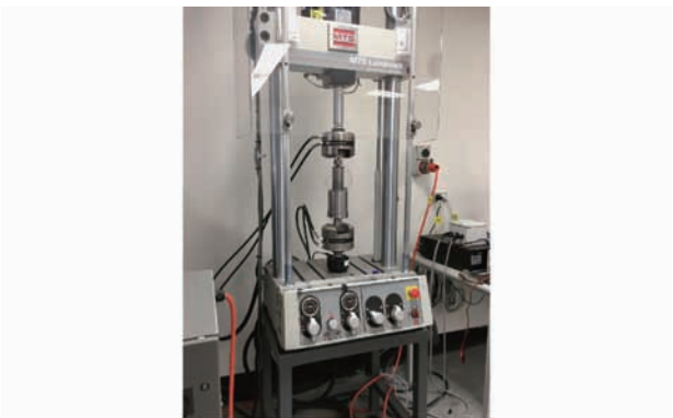
图 9 功能集成型阻尼器性能测试试验台 Fig.9 Test rig of multi-functional MR damper
