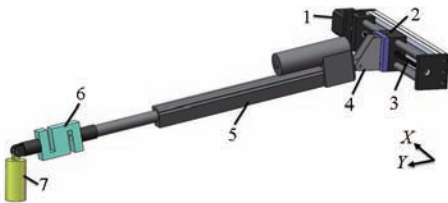
Fig. 3 Three-dimensional model of tractor driver robot's gear shift mechanical arm
