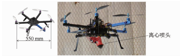
图 8 六旋翼无人机俯视图与离心喷头安装位置 Fig. 8 Top view of mini-UAV and installation site of spray nozzle
