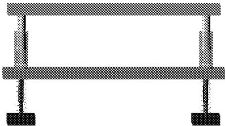
图 2 四自由度单桥连通式油气悬架多体动力学模型 Fig. 2 Multi-body dynamics model of 4-DOF signal-axis interconnected hydro-pneumatic suspension
